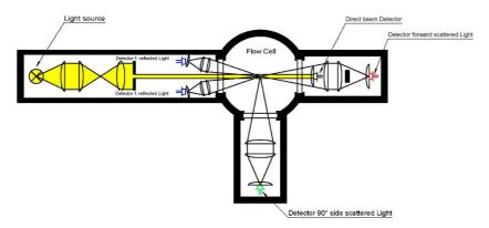
An intense collimated beam of light is projected through a sample contained within the sensor. The intensity of this light beam is measured by the direct beam detector, located opposite to the light source
